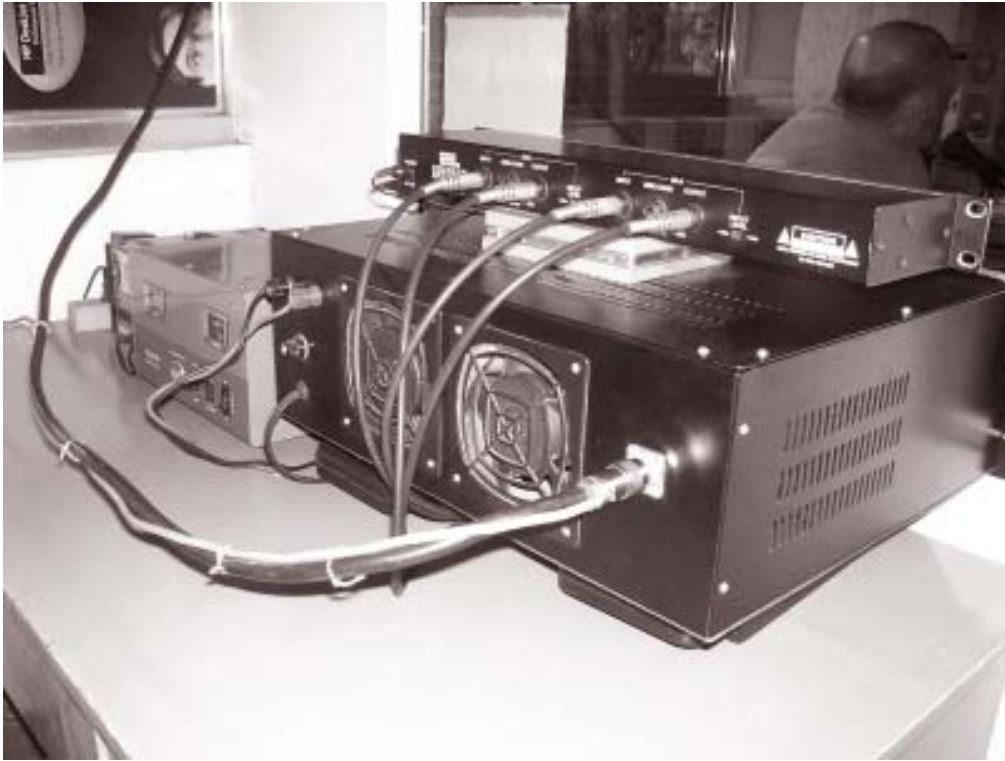
Low-power transmission equipment of DWEE. (LNT)
