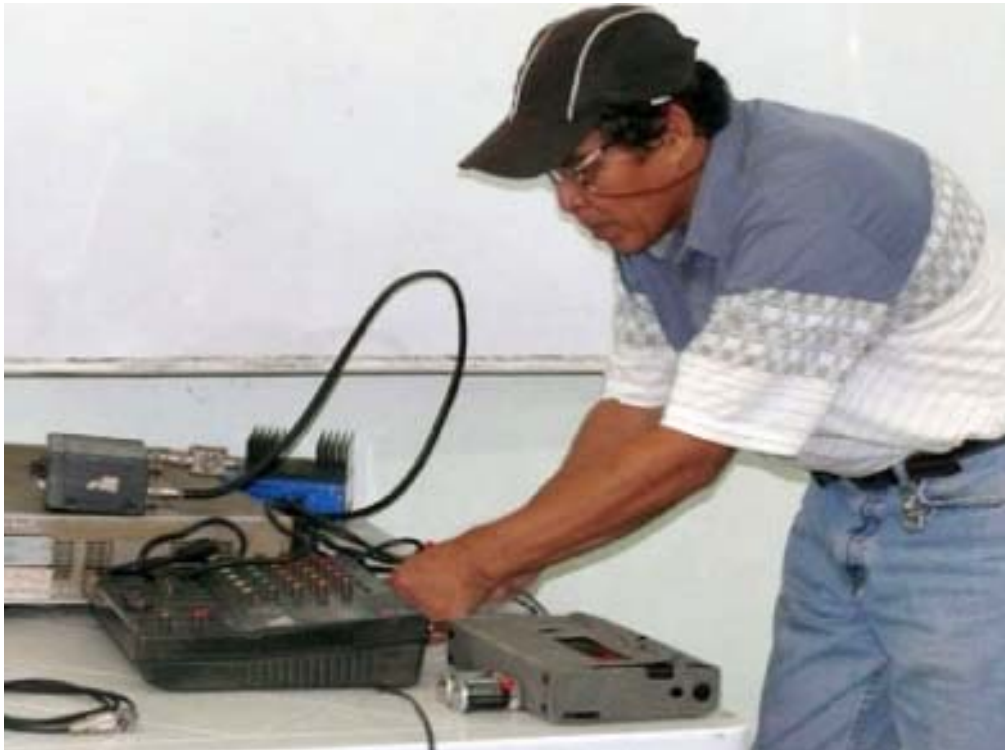
At St. John's Academy, General Trias, Cavite, Quiddie Labindao prepares the transmitter, antenna connection, power meter, mixer and audio cassette and microphone for test broadcast. (CAA)
